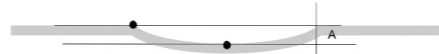
The deformation value is the height difference A between the two points shown
